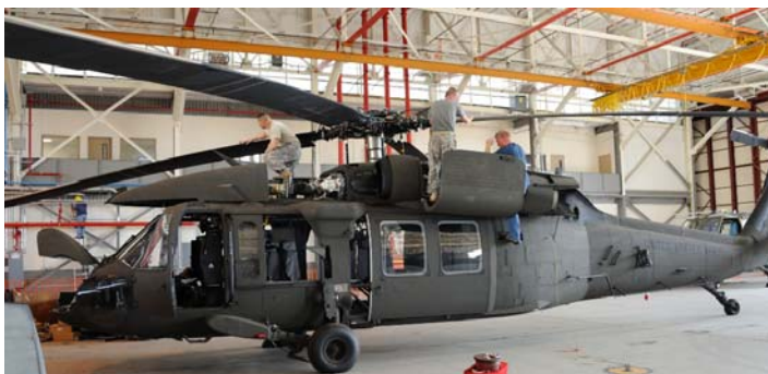
Corpus Christi Army Depot employees inspect a UH-60 Black Hawk during routine maintenance.
